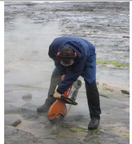
Heavy duty extraction with rock saw around the fossil site. Erich the Red Site (Otways) Photo: Lisa Nink
